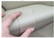
An example of holding your sample taut with your spray-out to maintain the same viewing angle and to keep the lighting the same. In this case, on the edge of the door panel. Finding an area of your repair you can keep taut can help, but this is not always necessary, especially if you cannot find a way to do it. Remember that perfect is often the enemy of great.
